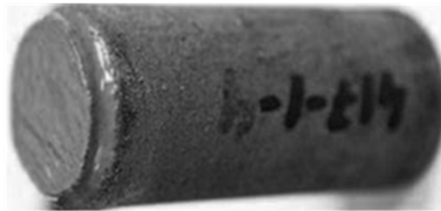
Fig. 5. Appearance of the core sample from Vyangapurovskoye oil and gas condensate field after dynamic and static tests on the FDES-645 unit
